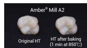
Stable translucency after baking of veneering
