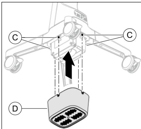
4. Loosen the four pre-mounted M4 x 10 screws (C) on the battery compartment (approx. 5 rotations).
