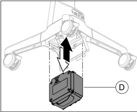
4. Pull the old battery (D) down out of the battery compartment and take it out of the unit.
