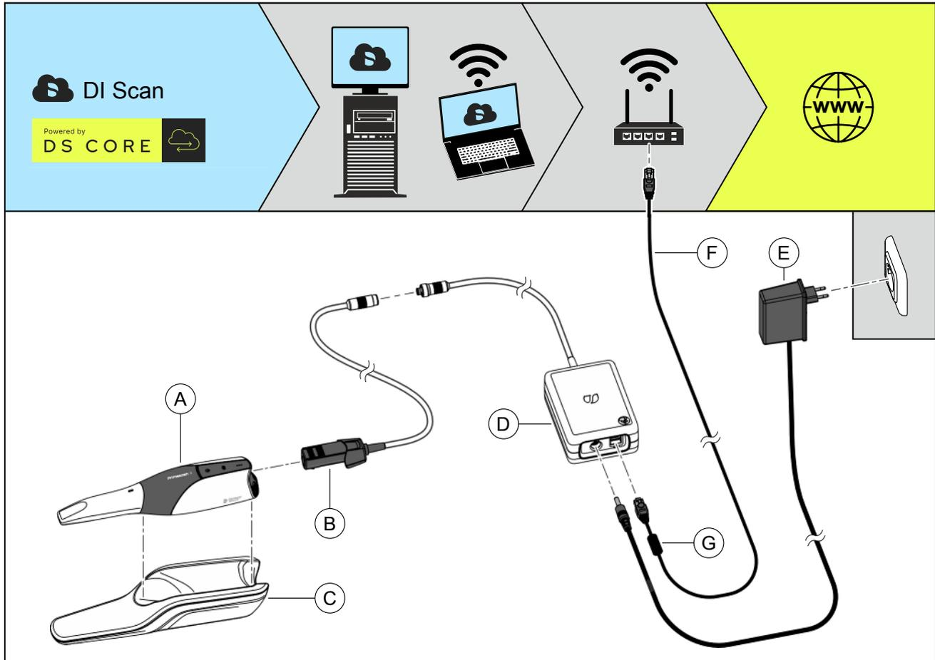
1. Guide the cable adapter (B) carefully into the scanner (A) until it clicks audibly into place.
