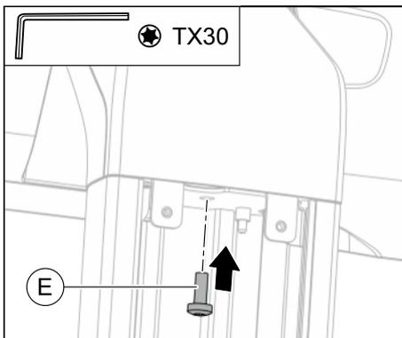
2. Screw the AIO monitor firmly onto the mobile stand using the included M6x16 screw (E).
