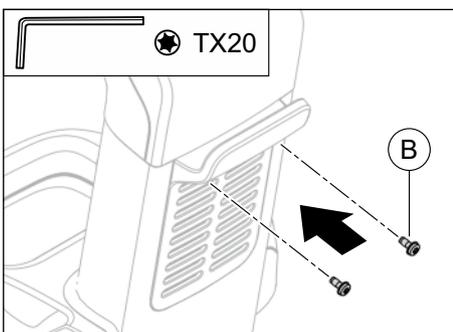
3. Screw the cover (A) firmly onto the mobile stand using the two included M4x10 screws (B) and washers. Use the included Torx TX20 offset screwdriver.
