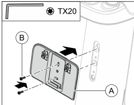
1. Place the wall holder (A) for the charger at the charger interface so that the two drill holes of the wall holder align with the drill holes at the interface.
