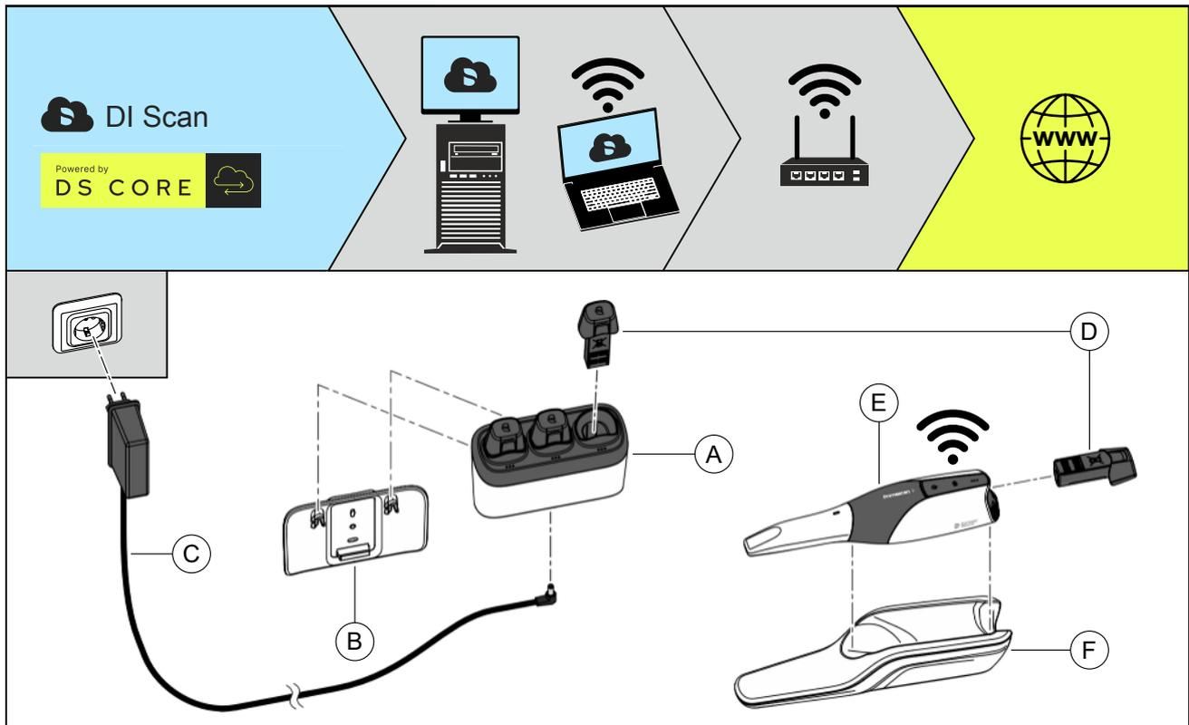
1. Insert the charger (A) into the wall holder (B) from above or place it on a flat surface outside the patient area.
