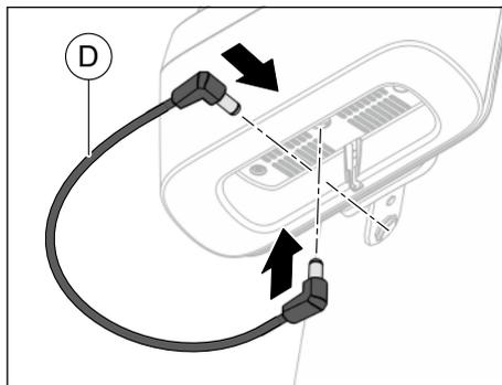
4. Connect the power connection of the charger to the power connection of the charger interface. Use the included power cable (D) with angled plugs.
