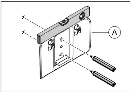
2. Hold the wall holder (A) at the desired mounting site and align it horizontally using a spirit level.
