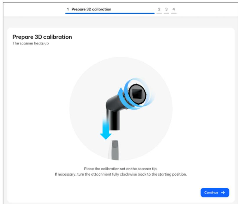
3. Secure the scanner in the calibration set using one hand. Ensure that the external calibration set screw is fully screwed in clockwise until it gently locks into place.
