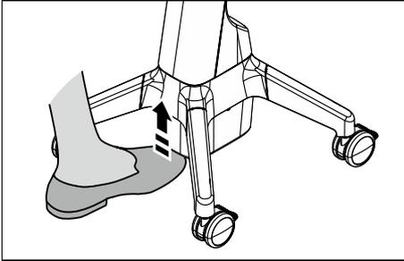
Press the battery cover upward with the tip of the foot to trigger the foot control.
