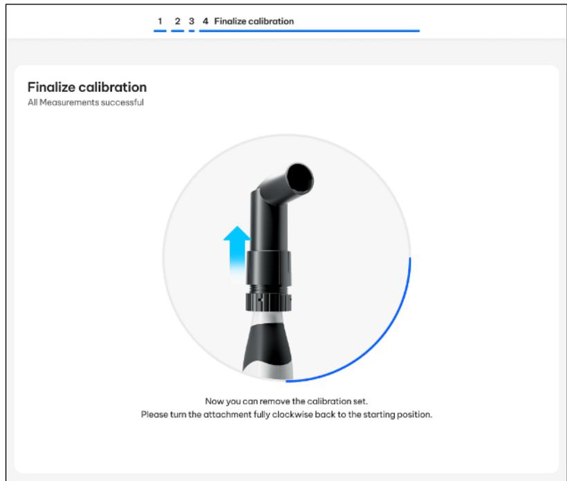
4. Take the calibration set off the tip of the scanner.
