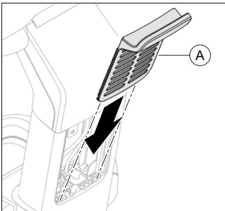
1. Set the cover (A) with the two flaps onto the lower edge of the recess of the mobile stand.
