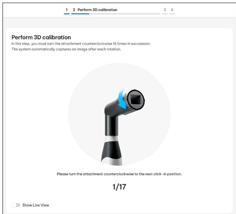
After the acquisition is made, you will be prompted to turn the screw of the calibration set to the next latching position.
