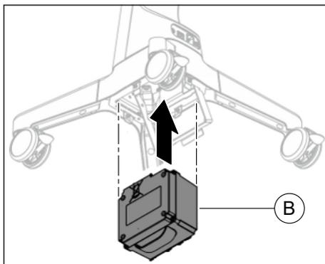
2. Insert the battery (B) from below with the electrical connection facing upward into the battery compartment as far as it will go.
