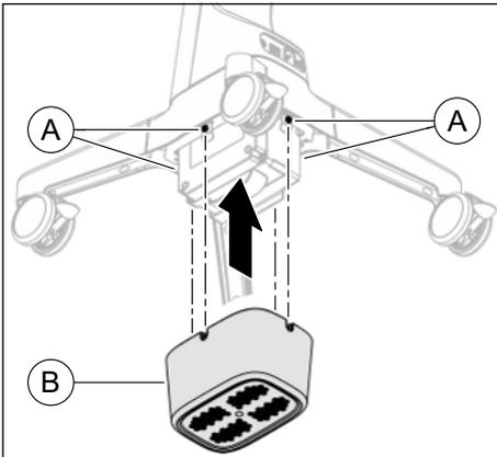
7. Slide the battery cover (B) onto the four pre-mounted screws (A).
