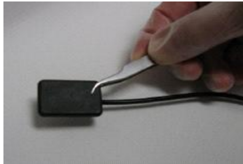
Do not use a clamp to hold sensor
