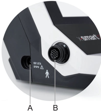
Fig. 4 Power and Motor handpiece connectors
