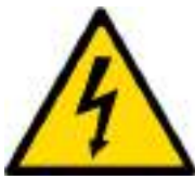
Warning; Electricity Code W012
