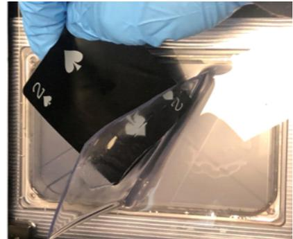
5. Lift the detached cleaning layer out of the vat and let the resin drip off over the vat.
