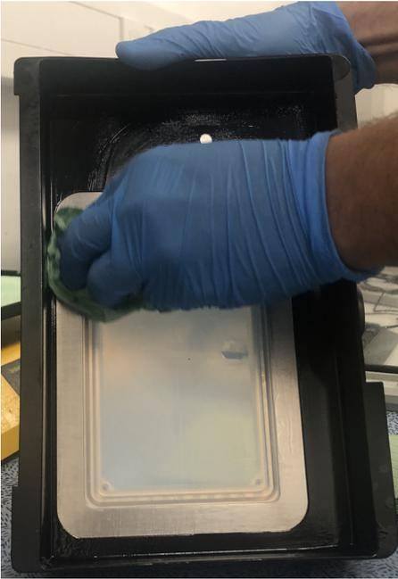
10. Wipe the vat with a clean cleaning cloth. Make sure that all resin residues are removed.
