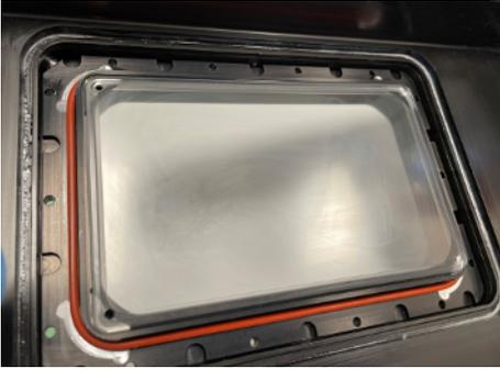
9. Remove the misty haze by buffing the window with a microfiber cloth and the supplied lens cleaner (it may take 1-2 minutes on each side for all of the misty haze to disappear).
