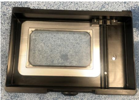
3. Position the conditioning unit perpendicular to the clamping frame with the left side of the conditioning unit flush with the right side of the clamping frame.
