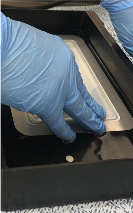
7. Remove the resin residues by rubbing the entire vat floor with your fingers until no more residue sticks to the vat floor.
