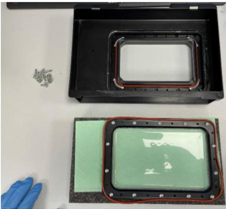
4. Carefully lift the vat so that the film clamp remains on the mounting aid. You may find that the film clamp is still somewhat stuck to the vat, so tap lightly to loosen it. Then turn the vat over. In addition to the film clamp, the outer sealing ring usually falls out as well.
