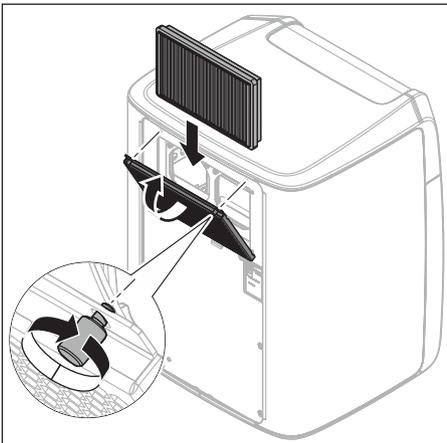
3. Insert a new activated carbon filter (REF 6747823).
