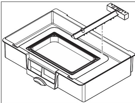
2. Pay attention to the orientation of the conditioning unit in the material unit vat. The bars must point toward the bottom and the rollers must point toward the rear.
