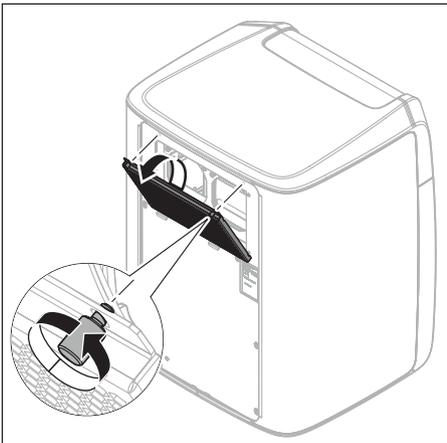
1. Before putting the unit in its place, insert the supplied activated carbon filter.
