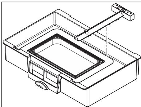
1. Pay attention to the orientation of the conditioning unit in the material unit vat. The bars must point toward the bottom and the rollers must point toward the rear.
