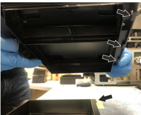
4. After the conditioning unit has been inserted, the cover of the material unit is now reconnected to the vat. For this purpose, the 3 latching hooks of the cover must engage in the edge of the vat.
