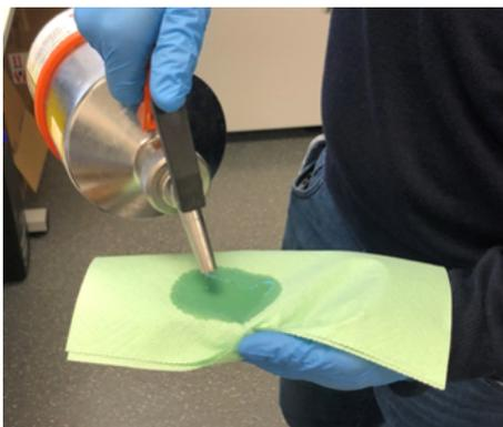
2. In addition, clean the build platform with a paper towel moistened with a little isopropanol.
