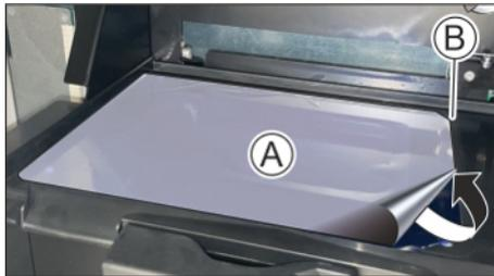
1. Before inserting it, remove the covering foil (A) from the heater plate (B), starting at the front corner.
