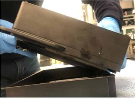
5. First hook the cover in at the back and then fold the cover down at the front.
