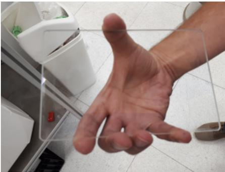
5. When inserting the window, make sure to touch the window only at the edges to avoid contamination. Carefully insert the window into the heater plate.
