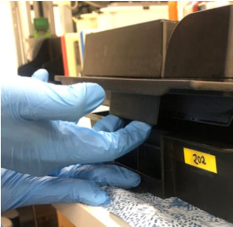
2. With the other hand, fix the vat so that you can fold the cover up and away.
