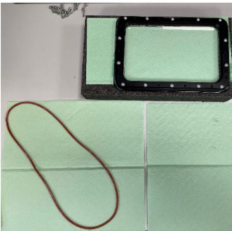
5. Separate the sealing ring from the clamping frame, if not already separated.
