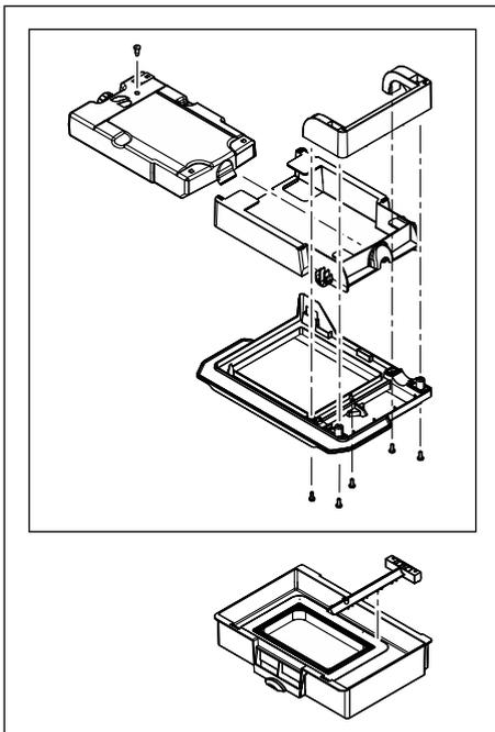
In order to clean the vat, replace the film insert or remove the conditioning unit, the cover of the material unit must be removed so that you have free access to the vat. Always wear gloves during all steps of the vat cleaning process to protect yourself and to keep the film grease-free.
