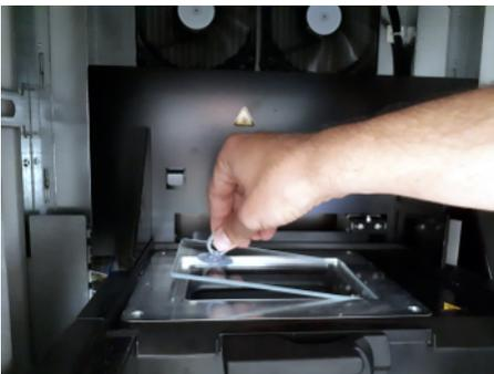
1. To clean the whole window, remove it from the heater plate. Use one of the supplied suction cups (REF 6810506) for this purpose.
