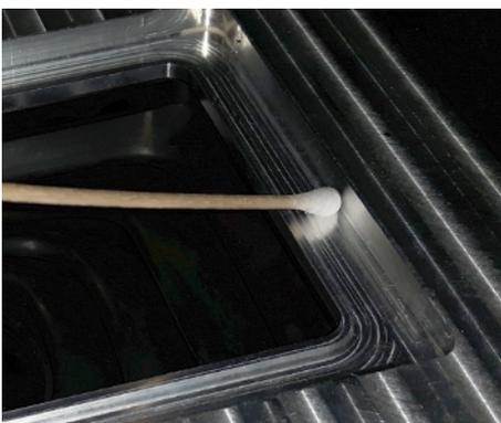
If resin gets in the groove under the window, wipe it away with isopropanol and a cloth or the enclosed cotton swab.
