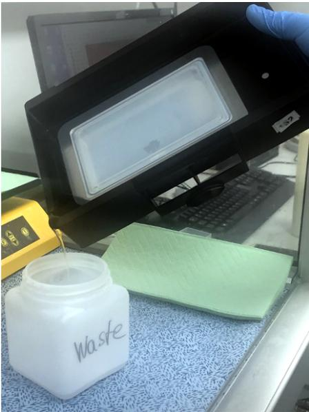
9. Empty the isopropanol with the residual resin from the vat into a resealable disposal container provided for this purpose.
