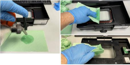
8. Clean possible resin residues on the window with a paper towel and some isopropanol. Isopropanol leaves a misty haze on the glass.
