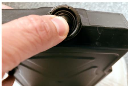
6. The valve must be pressed in once to relieve the outlet valve for the first time. To do this, stand the cartridge upright and briefly press the valve in.
