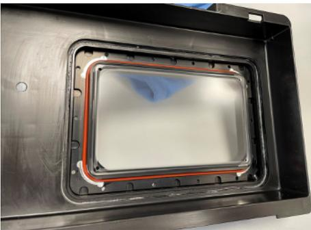
10. Insert the cleaned sealing ring into the recess. Ensure the clean and even fit of the sealing ring.
