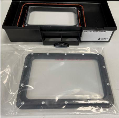
2. Carefully place the new film clamp in the vat. Make sure that the sealing ring underneath does not slip.
