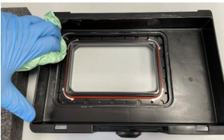
7. Clean the recess of the sealing ring with paper towels. Watch out for the glass!
