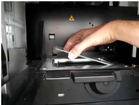
4. Insert the window into the corresponding cutout of the heater plate.
