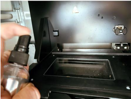
1. If there is resin residue on the window, clean it with a paper towel and isopropyl alcohol. Then wet the supplied microfiber cloth with the supplied lens cleaner and wipe over the glass pane. Then check the cleanliness of the glass pane in the installed state.
