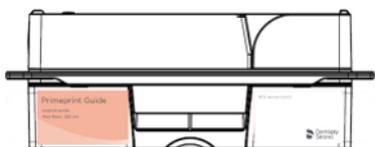
4. For visualization, you can apply the color-coded sticker included with the cartridge to the left vat side of the material unit. This is done to make it easier to relocate materials in the material cabinet.
